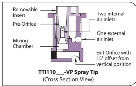
**Note:** Due to pre-orifice design, this tip is not compatible with the 4193A check valve tip strainer.
