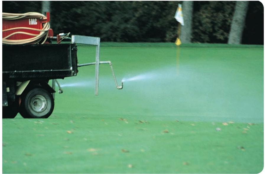
The KLC FieldJet nozzle is typically used to spray areas not accessible with a boom sprayer. Its one-piece nozzle design projects spray to both sides to form a wide swath flat spray. The round orifice minimizes clogging. Uniformity across the swath is not as good as with a properly operated boom sprayer.\* Available in brass or stainless steel.
