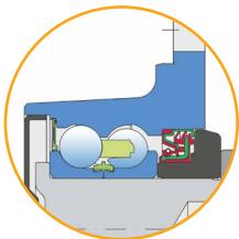
Sheet metal shield + RS seal/Dirtblock seal+ Forged cover plate
