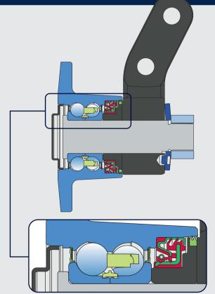
SHEET METAL SHIELD + RS SEAL / RS SEAL + DIRTBLOCK SEAL + DOUBLE LIP SEAL + FORGED COVER PLATE
